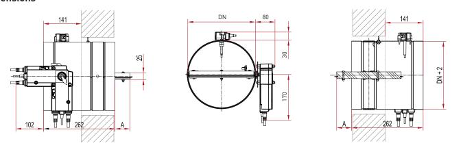
Figure 1. KTM-E-...-M damper (with a spring return actuator, sleeve connections).
