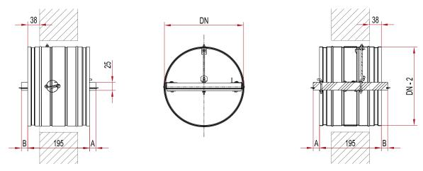
Figure 4. KTM-...-N damper (with a spring mechanism, nipple connections).
