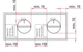
Figure 6. Spacing required between the dampers.
