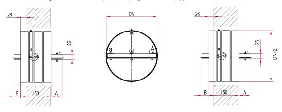
Figure 3. KTM-...-M damper (with a spring mechanism, sleeve connections).
