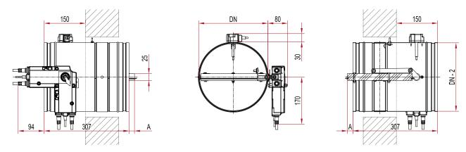
Figure 2. KTM-E-...-N damper (with a spring return actuator, nipple connections).
